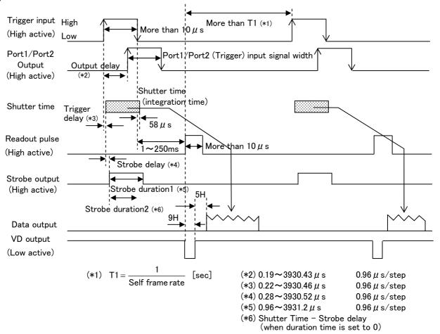
Note: Special function of reset control Trigger
