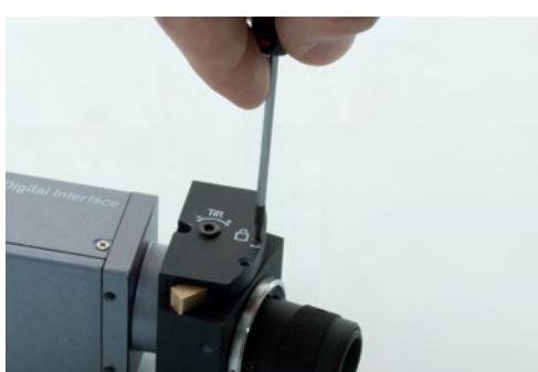
Setting-up the Scheimpflug mount is easy. First screw the lens into the camera C-mount, just like with any common lens. Loosen the lens C-mount adaptor by unscrewing the set-screws. Tune the lens phase to the right position, then tighten the set-screws.
