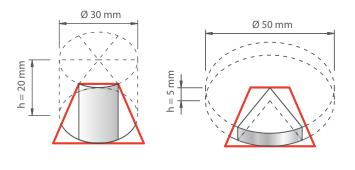
When the object height is maximum (20 mm) up to 30 mm diameter objects can be inspected
