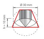
Combined view of both the inner sides and the bottom of a cavity possible up to 30 mm diameter and 10 mm height.
