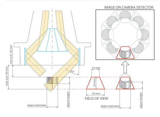
The diagram below shows how PolyView Optics image a cylindrical object. The object is observed at a 45° viewing angle, from 8 different points of view. Eight different trapezoidal Fields of View are obtained: all the object features included in such a trapezoid will be imaged on the corresponding image portion.
