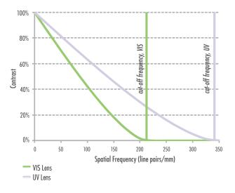
The graph on the left shows the limiting performances (diffraction limit) of two lenses operating at working F-number 8.
