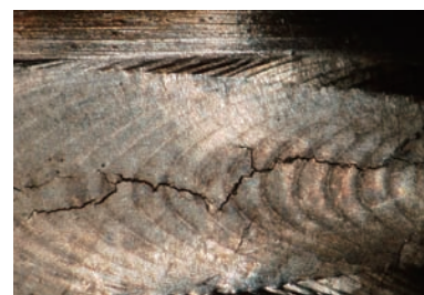
Section Fatigue Crack (50x)
